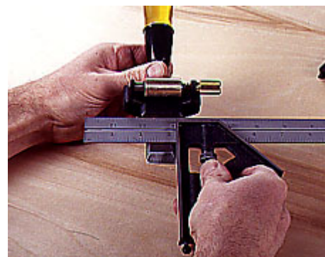
3—Check that the chisel is perfectly square to the edges of the honing guide, using a combination square.
