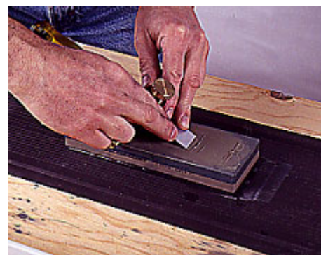
4—Place the chisel and guide on the coarse side of the stone and lightly move the blade back and forth.
